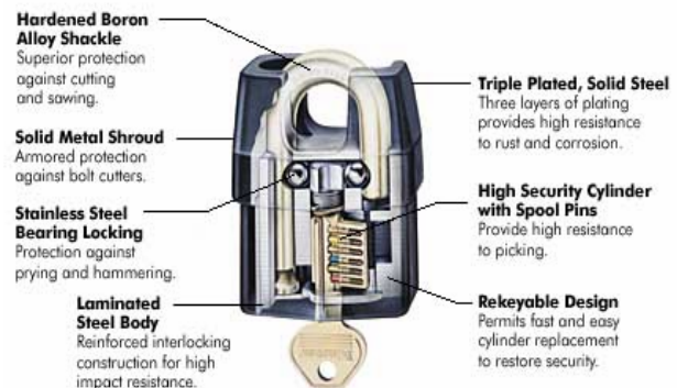
FIGURE 4-3 Example of a Tamper-proof, Shackle-protected Lock
